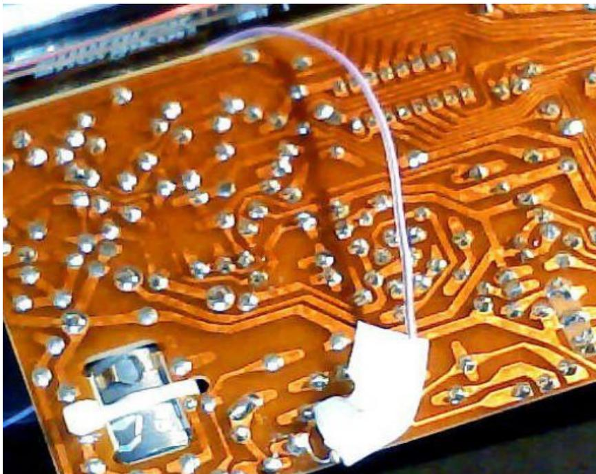
*Illustration 6: Insulating the resistor*
